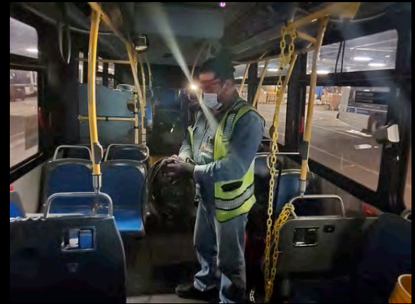
Preparing electrical and communication cables for OMNY retrofit on bus
