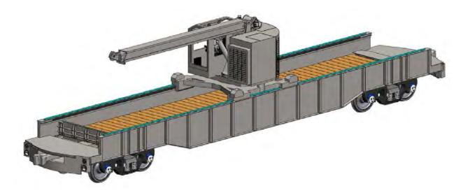
A rendering of the R253 crane car submitted for approval in this month's Board package is pictured above. Crane cars are used to perform lifting and placement of all track components such as rail, ties and other track-related equipment, and are an integral part of the NYCT's Track Maintenance Program.
