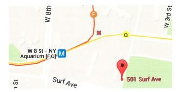
The average  $L_{EQ}$  for the F trains on the Jamaica-179<sup>th</sup> street bound track measured at the "X" on the above map is 85.1 dB(A), with an average  $L_{MAX}$  of 94.6 dB(A). The highest  $L_{EQ}$  measured was 87.8 dB(A) and the highest  $L_{MAX}$  measured was 97.1 dB(A). The F train produces elevated peaks on the 400 Hz, 500 Hz, 2kHz, and 6.3kHz bands during screeching.
