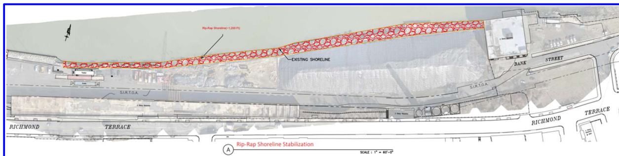
Figure 5: This plan has been developed to repair the eastern half of the Atlantic shoreline to preserve terminal space and to resist the erosion caused by strong tidal forces and heavy ship and tugboat traffic in the Kill Van Kull.
